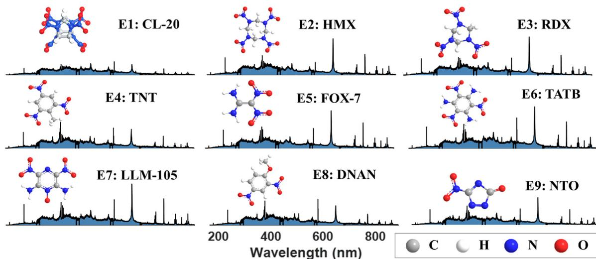
Fig. 2 LIPS spectra and molecular structures of HEs utilized in this work.
