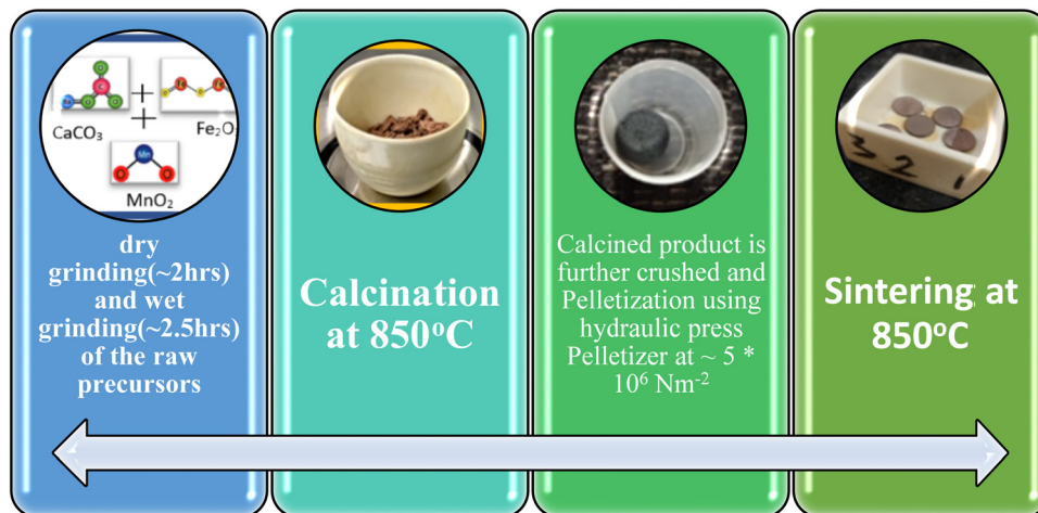
Fig. 1 Schematic diagram of the sample preparation method.
