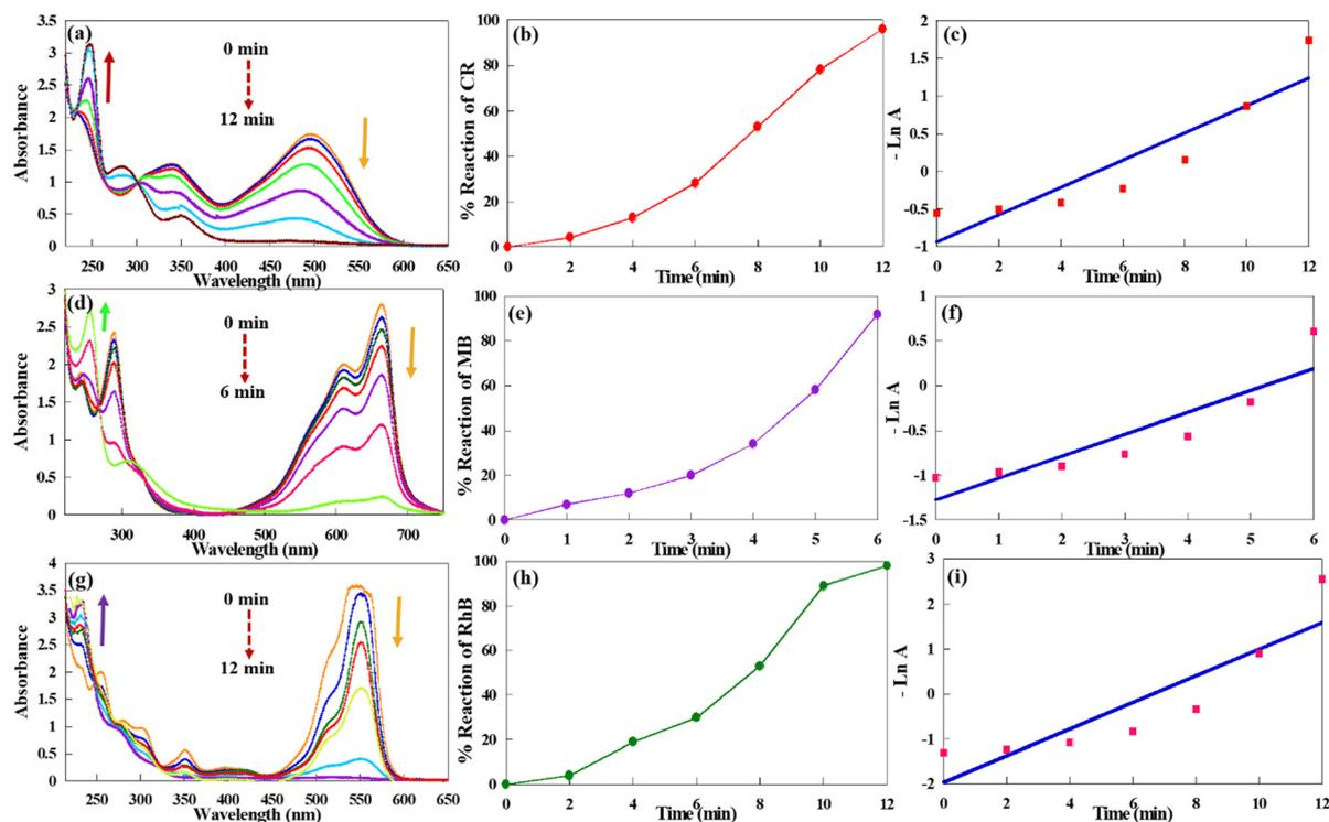
Fig. 8 The UV-vis spectra for the catalytic reactions of (a) CR at every 2 min, (d) MB at every 1 min, and (g) RhB at every 2 min; the reactions percent of (b) CR, (e) MB, and (h) RhB; and  $-\ln A$  versus time plots of (c) CR, (f) MB, and (i) RhB reactions for the kinetic examination.
