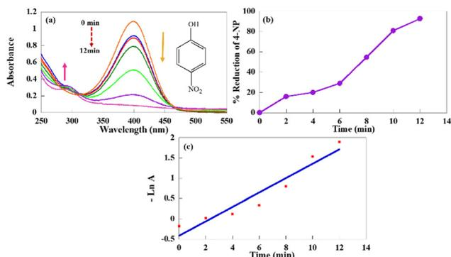
Fig. 4 (a) The UV-vis spectra for the reduction of 4-NP with NaBH<sub>4</sub> at every 2 min in the presence of CuPOM@melamine as the catalyst at room temperature, (b) the reduction percent of 4-NP, and (c)  $-\ln A$  versus time plot for the kinetic examination.
