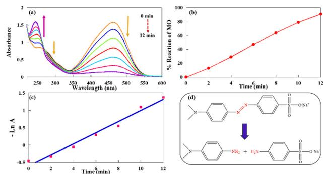
Fig. 7 (a) The UV-vis spectra of the MO catalytic reduction with  $\text{NaBH}_4$  using CuPOM@melamine at every 2 min. (b) The reduction percent of MO, (c) The plot of  $-\ln A$  versus time for the kinetic examination, and (d) The possible reduction reaction of MO.
