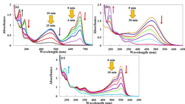
Fig. 10 The UV-vis spectra for the catalytic reactions of (a) MO and MB, (b) MO and CR, and (c) CR and RhB at room temperature.
