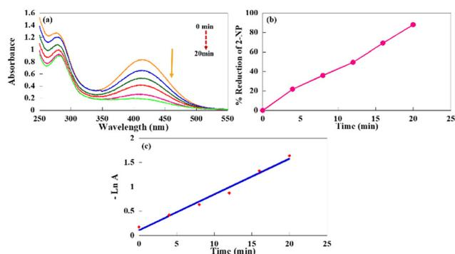
Fig. 5 (a) The UV-vis spectra for the reaction of 2-NP at every 4 min in the presence of CuPOM@melamine under optimized conditions. (b) The reduction percent of 2-NP, and (c)  $-\ln A$  *versus* time plot for the kinetic examination.
