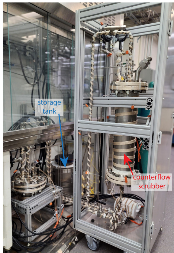
Fig. 2 Molten hydroxide (NaOH-KOH eutectic) showing interior before insulation. The external salt storage tank is shown on the left. This figure was modified from the original by McFarlane et al. 89 and reprinted with permission.
