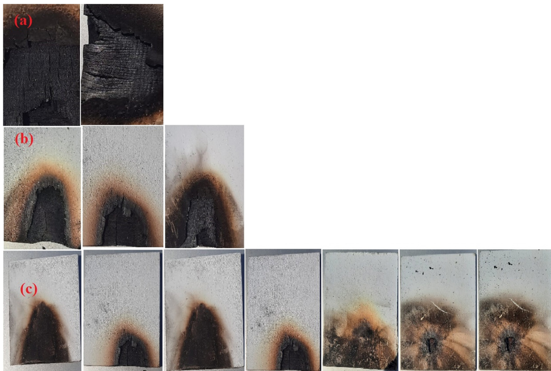
Fig. 7 Wood samples after the fire resistance test: (a) pure wood samples; (b) wood samples treated with paint; (c) wood samples coated with paints of mixed powders: 10wt%Al 2 O 3 and 10wt%Al 2 O 3 /5wt%Y 2 O 3 /xwt%GNSs (x: 0, 0.5, 1.0, 1.5, 2.0, 2.5), respectively.
