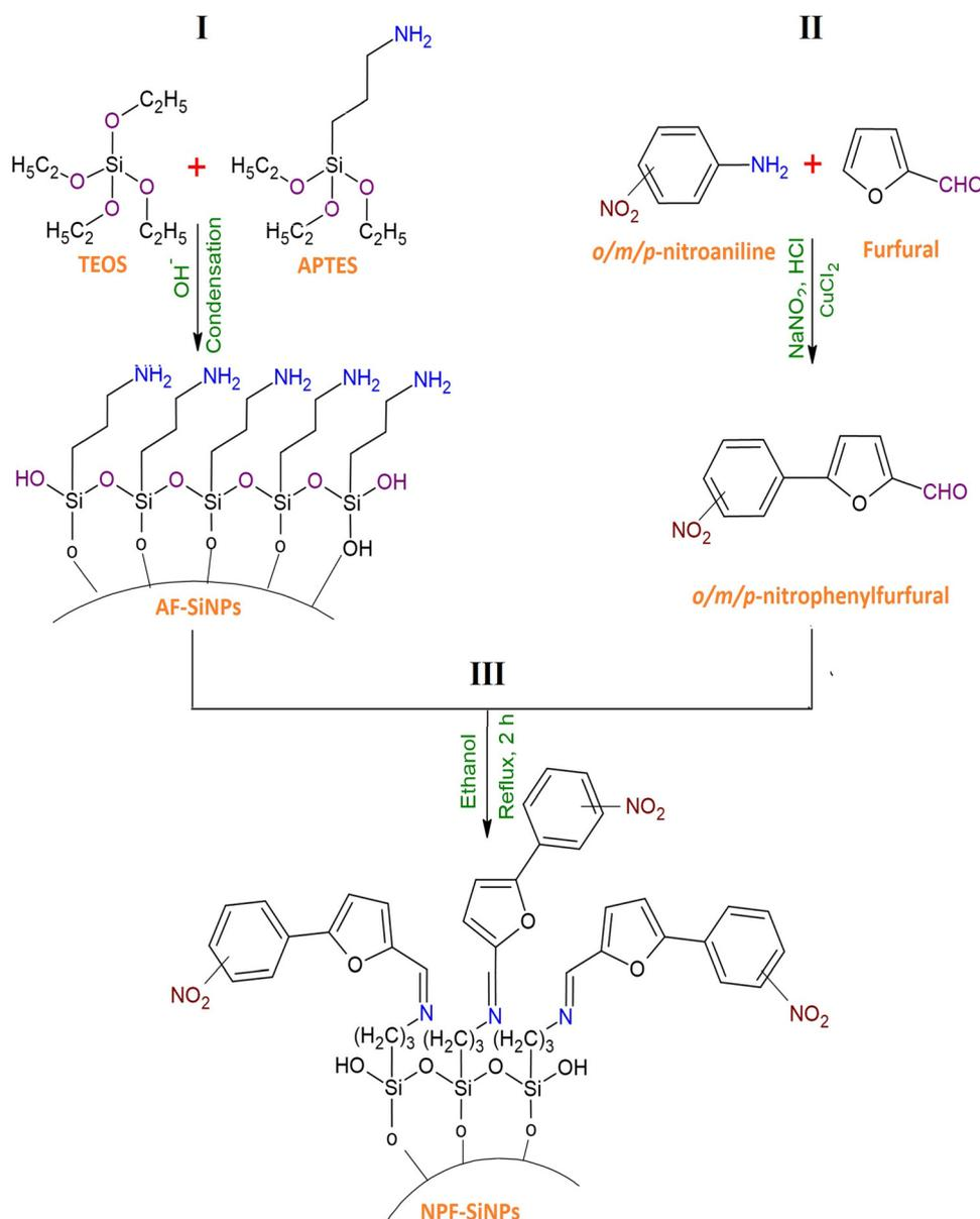
Scheme 1 (I) Synthesis of AFSi-NPs, (II) synthesis of *o/m/p*-nitrophenylfurfural, and (III) synthesis of NPF-SiNPs.
