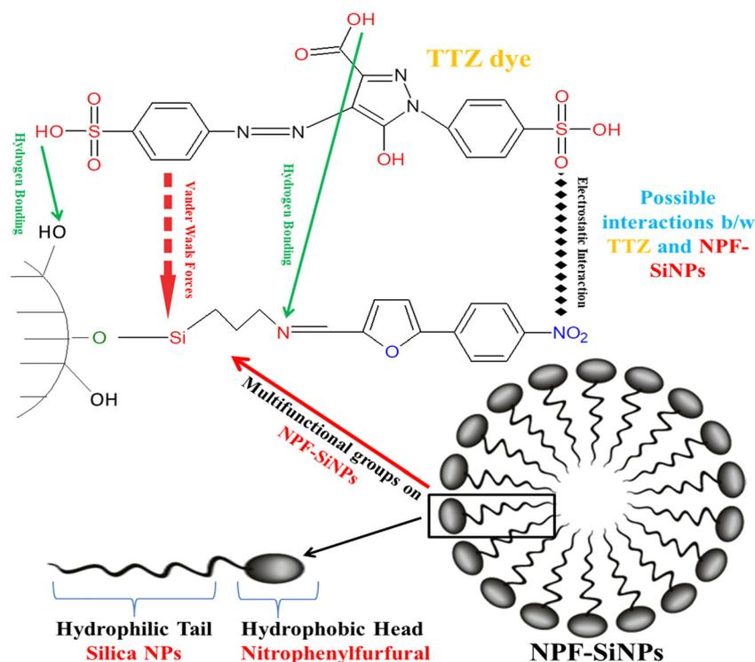
Scheme 3 Mechanism of micelle formation and TTZ interactions with NPF-SiNPs.
