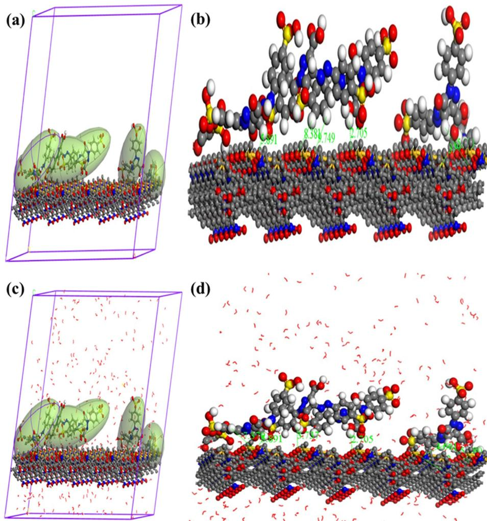
Fig. 9 The lowest-energy configurations of the TTZ molecule on the *p*-NPF-SiNPs' surface under dry condition (a) and (b) and MD images of the TTZ molecule being adsorbed on the *p*-NPF-SiNPs' surface in water (c) and (d). For clarity, TTZ is presented in polyhedron form and the bond length is given in angstroms.
