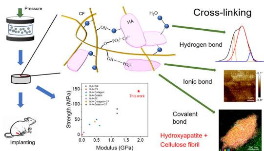
**Intensified cross-linking dramatically improved the mechanical properties of hydroxyapatite and cellulose composites for repairing bone segmental defects**
