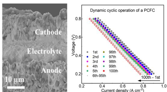
**A robust protonic ceramic fuel cell with a triple conducting oxygen electrode under accelerated stress tests**
