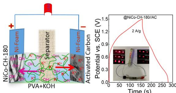
**Morphology-controlled synthesis of a NiCo-carbonate layered double hydroxide as an electrode material for solid-state asymmetric supercapacitors**
