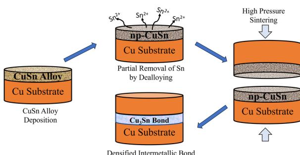
**New generation copper-based interconnection from nanoporous CuSn alloy film sintered at low temperatures**
