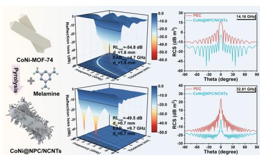
**N-doped branched metal–organic framework derivatives to boost multiband microwave absorption with ultrathin thickness**
