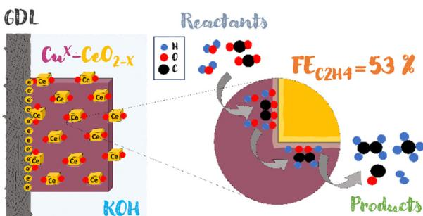
**CeO<sub>2</sub>-promoted Cu<sub>2</sub>O-based catalyst sprayed on the gas diffusion layer for the electroreduction of carbon dioxide to ethylene**
