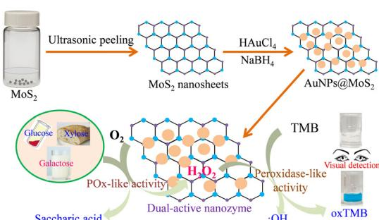
**Gold nanoparticle-loaded  $MoS_2$  nanosheets with peroxidase-like and pyranose oxidase-like activities for bio-enzyme-free visual detection of glucose, xylose and galactose**
