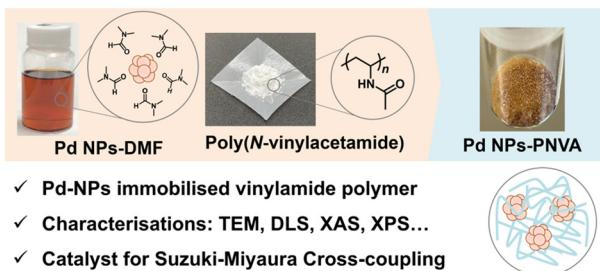
**Synthesis of colloidal Pd nanoparticles immobilised on poly(*N*-vinylacetamide): characterisation and application in catalysis**
