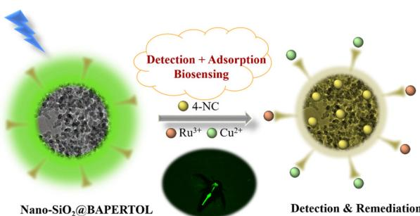
**Perylene diimide functionalized nano-silica: green emissive material for selective probing and remediation of 4-nitrocatechol, Ru<sup>3+</sup>, and Cu<sup>2+</sup> with biosensing applications**
