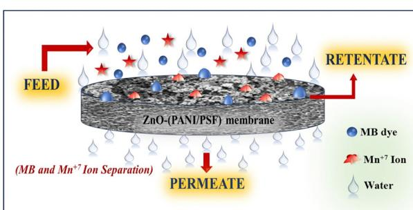
**Enabling improved PSF nanocomposite membrane for wastewater treatment with selective nanotubular morphology of PANI/ZnO**
