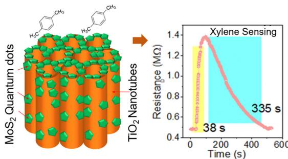
**A MoS<sub>2</sub> quantum dot functionalized TiO<sub>2</sub> nanotube array for selective detection of xylene at low temperature**
