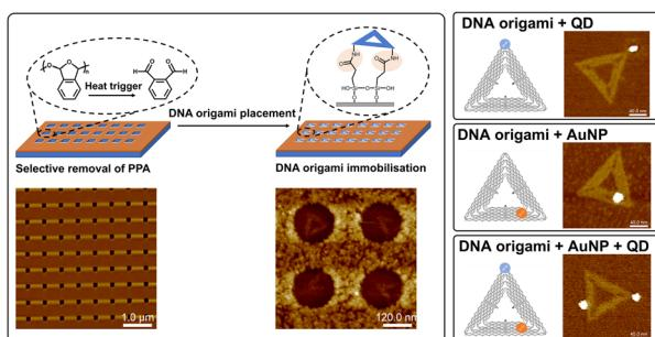
**Selective placement of functionalised DNA origami via thermal scanning probe lithography patterning**
