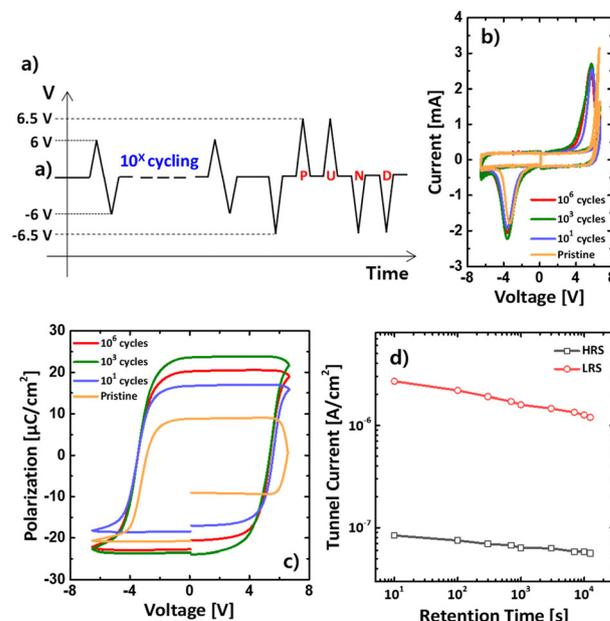
Fig. 8 Pulse scheme for stress cycling (a). Changes of polarization switching currents extracted by PUND measurement with respect to the number of cycling (b) and the corresponding  $P$ - $V$  curves (c). Retention characteristics measured at 30 °C after cycling (d).
