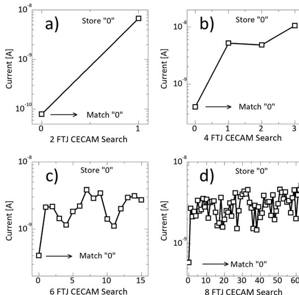
Fig. 10 Searching results of N-CECAM based on HZO FTJ ( $100 \times 100 \mu\text{m}^2$ ) crossbar arrays with same stored information of “0” with different N values:  $N = 1$  (a),  $N = 2$  (b),  $N = 3$  (c), and  $N = 4$  (d).
