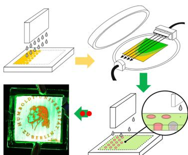
**Bicolour, large area, inkjet-printed metal halide perovskite light emitting diodes**
