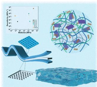
**An ultra-soft conductive elastomer for multifunctional tactile sensors with high range and sensitivity**
