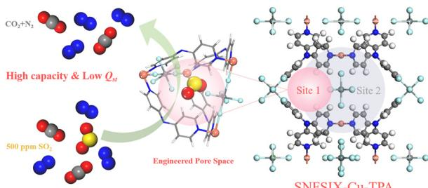
**Trace  $\text{SO}_2$  capture within the engineered pore space using a highly stable  $\text{SnF}_6^{2-}$ -pillared MOF**
