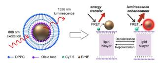
Voltage-sensitive Luminescence under the NIR-IIb window
