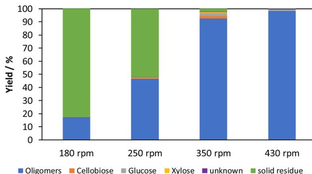
Fig. 10 Product composition after mechanocatalytic partial depolymerization by varying the rotational speed. Reaction conditions: 3% acid content, 20% filling level with tungsten carbide grinding balls, 85 min.
