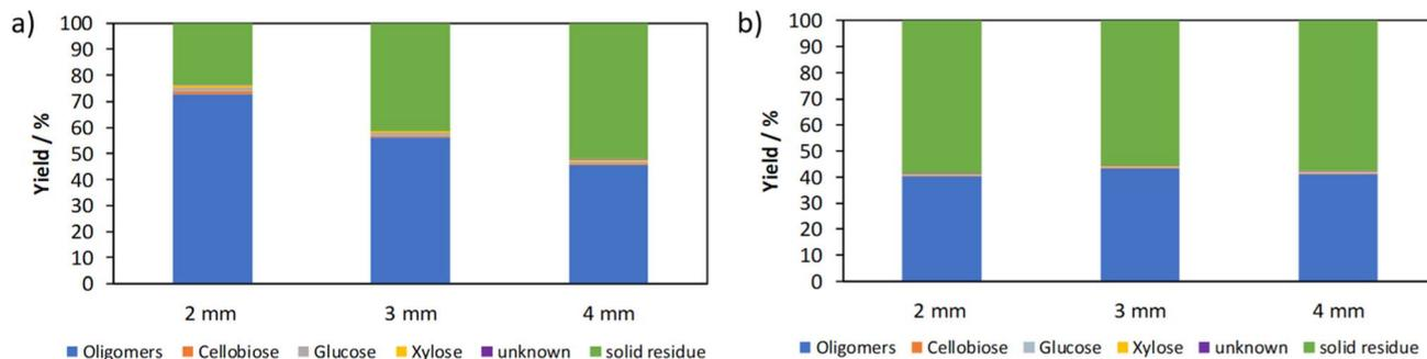
Fig. 9 Product composition after mechanocatalytic partial depolymerization with different grinding ball diameters: (a) 3% acid content, 20% filling level with stainless steel grinding balls, 430 rpm, 40 min. (b) 6% acid content, 20% filling level with stainless steel grinding balls, 350 rpm, 40 min.
