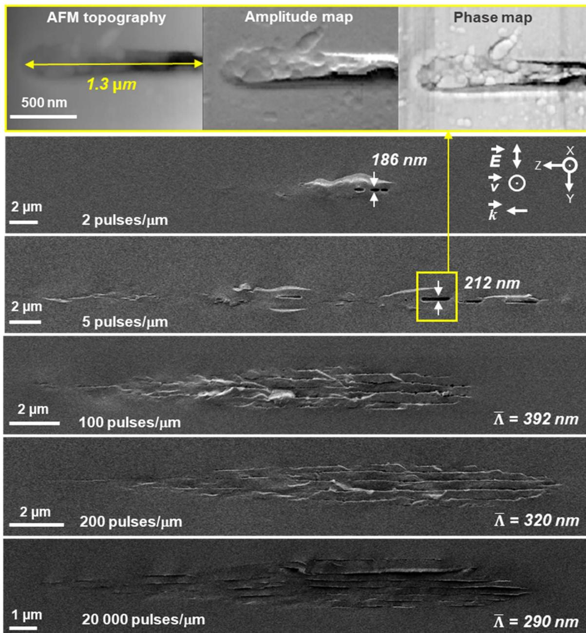
Fig. 6 AFM intermittent contact mode and SEM secondary electron images of laser track cross-section according to pulse density expressed in pulses per  $\mu\text{m}$ . The laser parameters were:  $0.5 \mu\text{J}$  per pulse,  $1030 \text{ nm}$ ,  $300 \text{ fs}$ ,  $0.6 \text{ NA}$ ,  $100 \text{ kHz}$  and  $Xy$  configuration.
