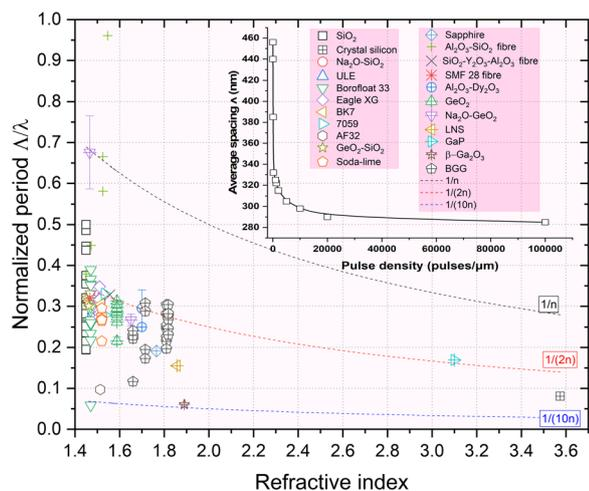
Fig. 7 Normalized period  $\Delta/\lambda$  of the overall investigated glasses in the literature including commercial glasses vs. refractive index,  $n$ , measured at 550 nm. The laser wavelength  $\lambda$  used in the various experiments was typically between 515 and 1030 nm. Data were extracted from the following ref. 17, 20, 23–26, 45, 48 and 54–67.
