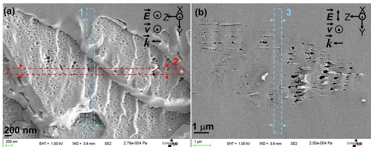
Fig. 2 SEM micrographs of (a) nanopores ( $Xx$  writing) and (b) nanoplanes ( $Xy$  writing). The red arrows in the  $Y$  direction and blue ones in the  $Z$  direction are the directions of FIB milling for TEM sample preparation (typical slice thicknesses are smaller than 50 nm). The numbers 1–3 correspond to the 3 slices extracted by FIB and subsequently observed.
