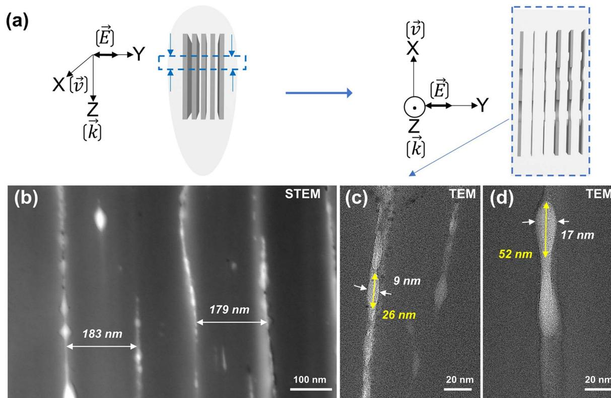
Fig. 5 (a) The schematic of the FIB milling process. (b) STEM and (c and d) TEM micrographs from Fig. 2(b) (nanoplanes) in blue arrows in XY plane observation. The writing configuration is  $Xy$ .
