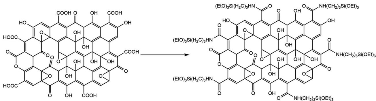
Scheme 1 Preparation of APTES-rGO from GO, drawing based on information in Aliyev *et al.*<sup>33</sup>
