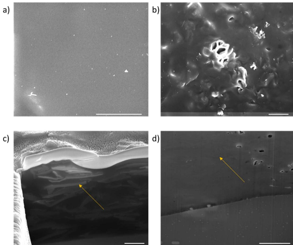
Fig. 11 Plan SEM views of the coatings. (a) APTES-rGO and (b) rGO, cross sectional views of the coatings (c) APTES-rGO and (d) rGO. The scale bar is 5  $\mu\text{m}$ .
