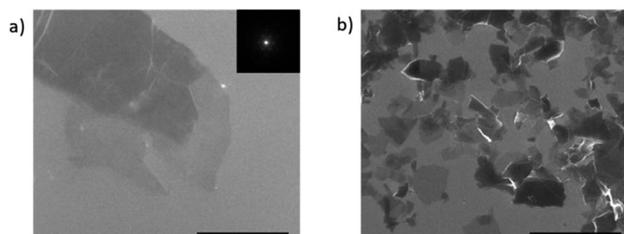
Fig. 5 SEM micrograph of (a) GO and (b) APTES-rGO. The indicated scale bar is 2  $\mu\text{m}$ .
