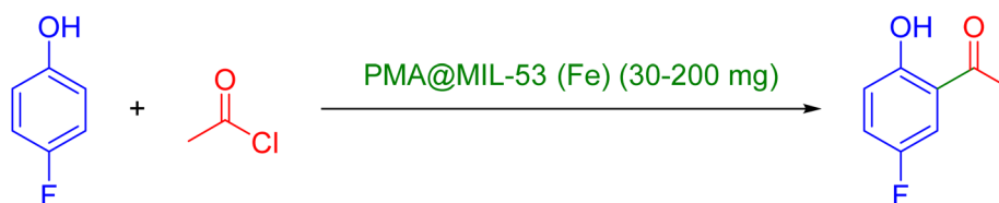
Scheme 2 Friedel–Crafts C -acylation of para -fluorophenol over the catalysis of PMA@MIL-53 (Fe) MOF.
