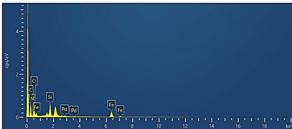
Fig. 11 EDS spectrum of the recovered  $\text{Fe}_3\text{O}_4/\text{GO-IL-Pd}$  catalyst.
