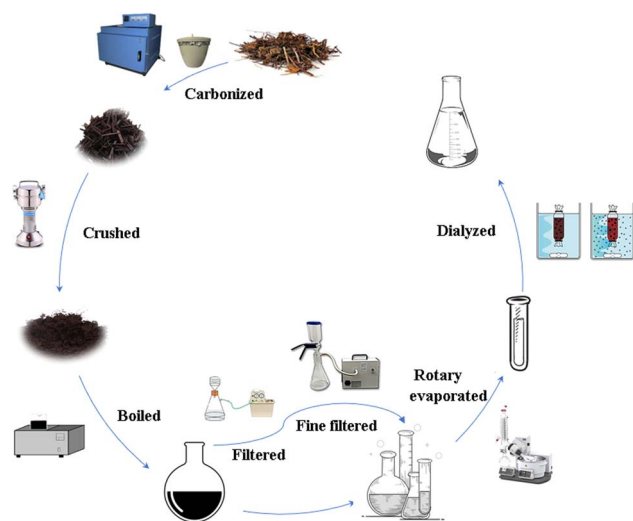
Fig. 1 Flow diagram of the preparation process of Rubia cordifolia L.-carbon dots (RCL-CDs).
