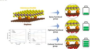
First-principles evaluation of transition metal dichalcogenide—graphene pairs functionalized with oxygen-containing groups for sodium-ion battery anodes
