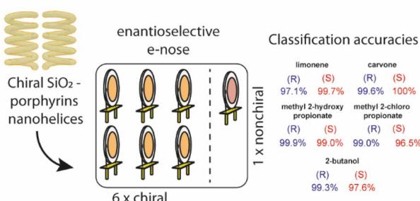
**Chiral porphyrin- $\text{SiO}_2$  nano helices-based sensors for vapor enantiomers recognition**
