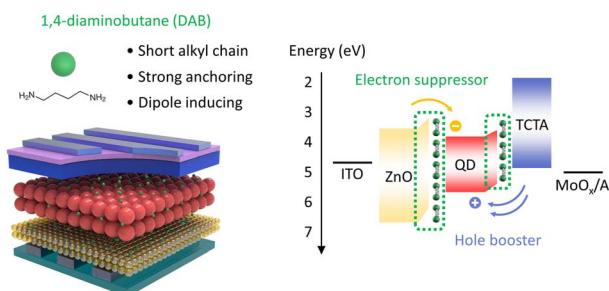
**Utilizing a compact diamino-based ligand as a charge balancer in quantum dot light-emitting diodes**
