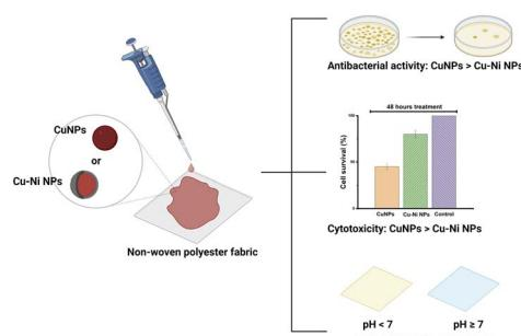
**Nickel coating on plasmonic copper nanoparticles lowers cytotoxicity and enables colorimetric pH readout for antibacterial wound dressing application**
