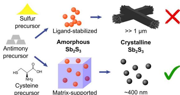
**Colloidal spherical stibnite particles via high-temperature metallo-organic synthesis**
