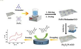
A catalytic amplification platform based on  $Fe_2O_3$  nanoparticles decorated graphene nanocomposites for highly sensitive detection of rutin
