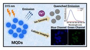
L-cysteine capped MoS<sub>2</sub> QDs for dual-channel imaging and superior Fe<sup>3+</sup> ion sensing in biological systems
