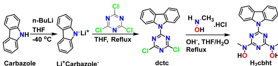
Scheme 2 Synthesis of organic molecules *dctc* and  $\text{H}_2\text{cbht}$ .
