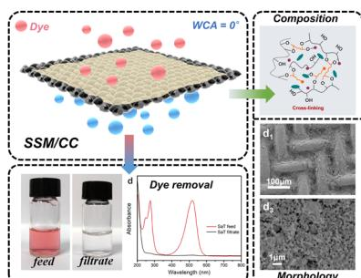
**Brushing a superhydrophilic cross-linked coating on the metal mesh for dye separation**
