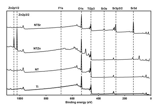
Fig. 3 XPS spectra of different surfaces.
