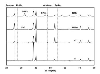
Fig. 5 XRD spectra of different surfaces.
