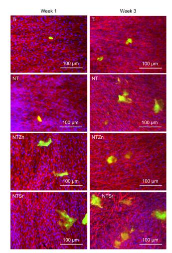
Fig. 12 Immunofluorescence microscopic images of the surfaces after 1 and 3 weeks of culturing ADSCs with differentiation media. The green color represents osteocalcin expression by the differentiated ADSCs.
