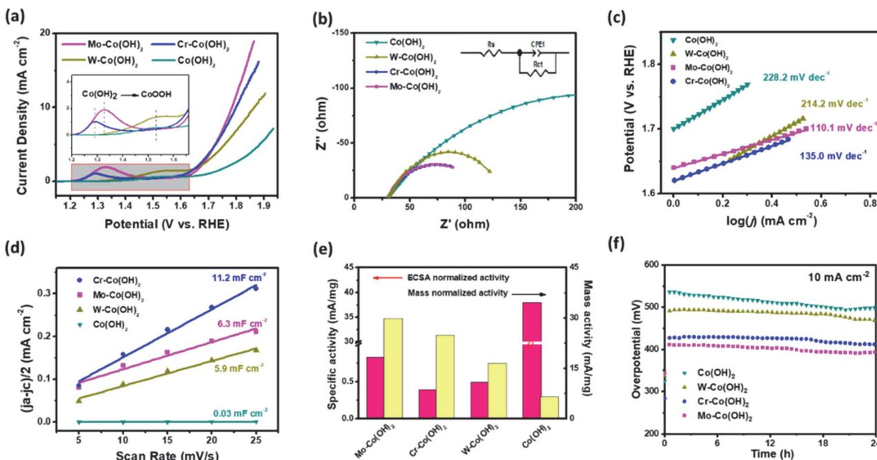
Fig. 2 (a) iR-corrected polarization curves of HVM-modified  $\text{Co}(\text{OH})_2$  during the OER. (b) Nyquist plots of the catalysts, and the inset shows the equivalent circuit mode. (c) Tafel plots of the different catalysts. (d) Double-layer capacitance plots of the different catalysts. (e) Specific activity normalized to ECSA and mass and (f) stability test of  $\text{Co}(\text{OH})_2$  and HVM-modified  $\text{Co}(\text{OH})_2$  under  $10 \text{ mA cm}^{-2}$ .
