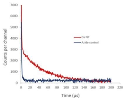
**Fig. 7** Time-resolved singlet oxygen NIR phosphorescence decays from **OsPhenSS-AuNP13** in  $D_2O$  4.5 nM ( $\lambda_{det} = 1270 \pm 20$  nm). Red: without the addition of azide; blue: with the addition of azide (5 mM). The initial short-lived signal is due to the residual NIR tail of fluorescence from the osmium signal. In the presence of azide, which is a physical quencher of singlet oxygen, the NIR phosphorescence tail is suppressed.
