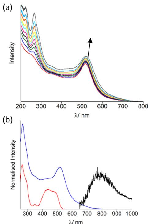
**Fig. 3** Monitoring **OsPhenSS** coating on AuNP13 and optical spectra of isolated **OsPhen-AuNP13** in water. (a) Titration of 5  $\mu\text{L}$  quantities of 1 mM **OsPhenSS** (5  $\mu\text{L}$  aliquots of 1 mM) into 4.5 nM Z-AuNP13 (4.5 nM) in aerated water and (b) isolated **OsPhen-AuNP13** UV-Vis absorption spectrum: blue, excitation spectrum ( $\lambda_{\text{em}} = 770$  nm); red, and luminescence emission spectrum ( $\lambda_{\text{exc}} = 488$  nm), black.
