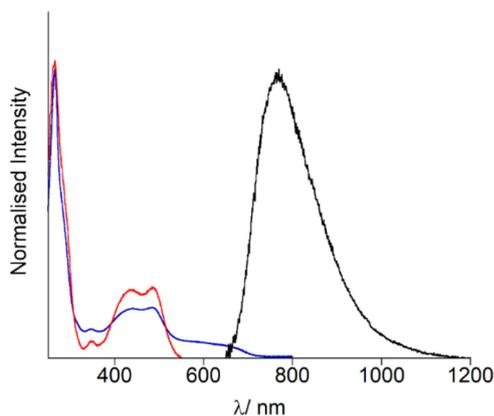
**Fig. 2** Optical spectroscopy of **OsPhenSS** in aerated aqueous solution (2% CH<sub>3</sub>CN) UV-Vis absorption spectrum: blue, luminescence excitation spectrum ( $\lambda_{\text{em}} = 770$  nm) red, and luminescence emission spectrum ( $\lambda_{\text{exc}} = 488$  nm); black.
