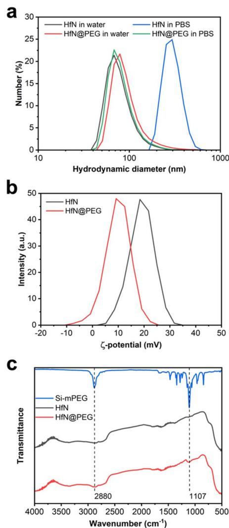
**Fig. 5** Coating of laser-synthesized HfN-based NPs with PEG. (a) Hydrodynamic diameter distribution for HfN and HfN@PEG NPs in water and PBS buffer. (b)  $\zeta$ -potential distribution for HfN NPs before and after coating with mPEG-Silane polymer. (c) FTIR spectra of mPEG-Silane polymer, HfN and HfN@PEG NPs.
