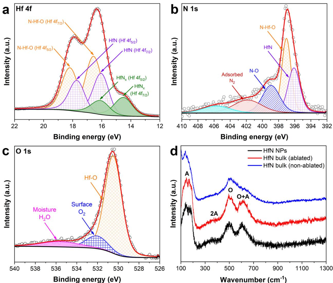
**Fig. 3** X-ray photoelectron spectroscopy (XPS) characterization of laser-synthesized HfN-based NPs from different parts of the spectrum: Hf 4f (a), N 1s (b), O 1s (c). The data are presented for a sample prepared in acetonitrile. Shirley background correction is applied. (d) Raman spectra of HfN-based NPs.
