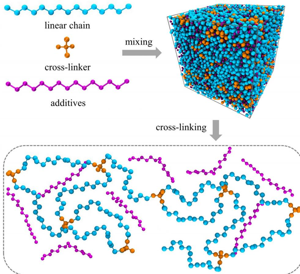
**Fig. 1** The molecular structures of linear chain (cyan beads), cross-linker (orange beads) and additive (purple beads). The molecules are homogeneously mixed in an amorphous simulation box with periodic boundary conditions. Subsequently, the linear chains and cross-linkers are cross-linked to a polymer network.
