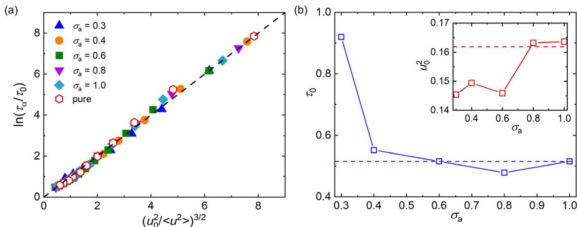
**Fig. 6** (a) Tests of the localization model predictions (dashed line) for pure polymer and polymer/additive mixtures with varying additives size  $\sigma_a$ . The data show a good collapse onto the localization model. (b) The fitting parameters  $\tau_0$  and  $u_0^2$  as a function of  $\sigma_a$ . The dashed lines are the fitting parameters of pure polymer.
