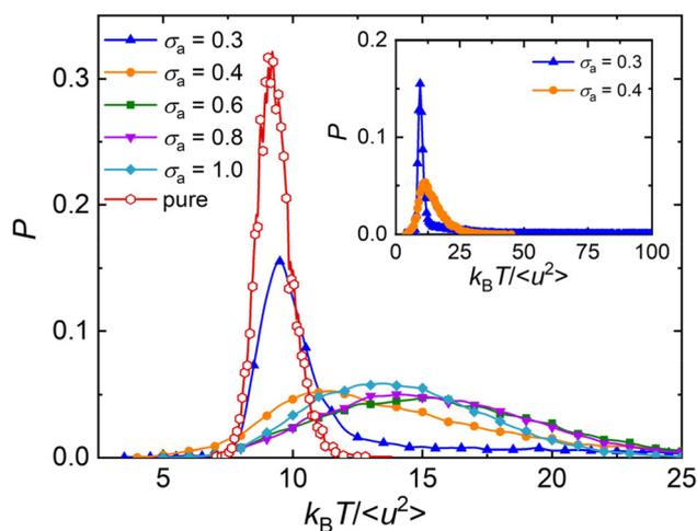
**Fig. 8** The probability density distribution of local stiffness  $k_B T / \langle u^2 \rangle$  at  $T = 0.5\epsilon/k_B$  for pure polymer and polymer/additive mixtures with varying additives size  $\sigma_a$ . The inset describes the entire distribution of  $k_B T / \langle u^2 \rangle$  for mixtures with  $\sigma_a = 0.3\sigma$  and  $\sigma_a = 0.4\sigma$ .
