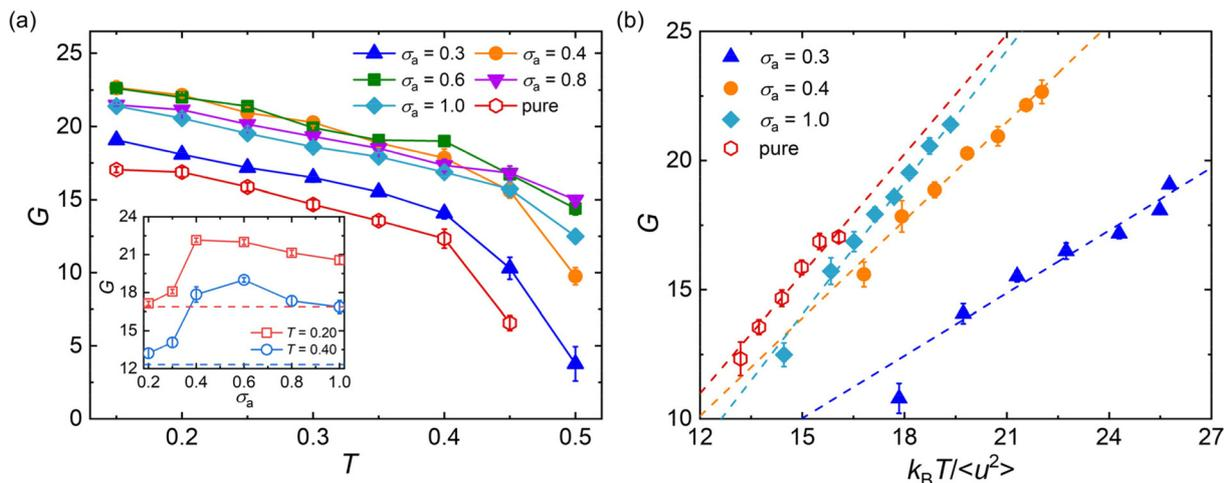
**Fig. 7** The glassy shear modulus  $G$  for pure polymer and polymer/additive mixtures with varying additives size  $\sigma_a$ . (a)  $G$  as a function of temperature  $T$ . The inset describes  $G$  as a function of  $\sigma_a$ . (b)  $G$  as a function of local molecular stiffness  $k_B T / \langle u^2 \rangle$ . The dashed lines indicate the linear fitting.
