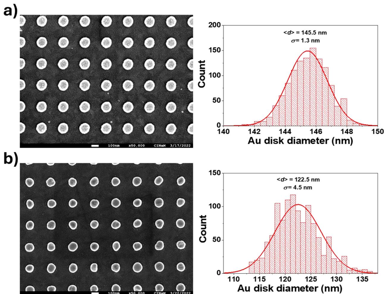
**Fig. 3** SEM images (same magnification  $\times 50\,000$ ) and disk diameter size distributions of Au disks ( $h = 17.5$  nm,  $p = 300$  nm) deposited onto an ITO-coated film (21 nm) glass window before (a) and after (b) annealing at 350 °C under He flow. SEM images were taken with a JEOL JSM-7900F.
