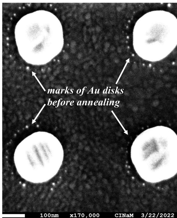
Fig. 4 High magnification ( $\times 170\,000$ ) SEM image of Au disks ( $h = 17.5$  nm,  $p = 300$  nm,  $d = 140$  nm) deposited onto an ITO-coated film (21 nm) glass window after annealing at  $350$  °C under He flow. The image was taken with a JEOL JSM-7900 F.
