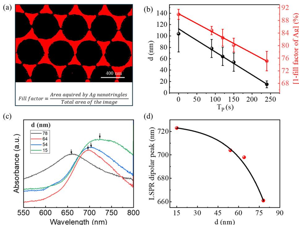
**Fig. 2** (a) Ag fill factor (FF) calculation from FESEM image. (b) Average nanogap ' $d$ ' and FF variation (shown as  $1 - \text{FF}$ ) with OPT time ( $T_p$ ), (c) absorption spectra of Ag superlattice structures prepared by following  $T_p$  of 90, 120, 150, and 240 s. (d) Variation of the corresponding LSPR dipolar peak with the nanogap.
