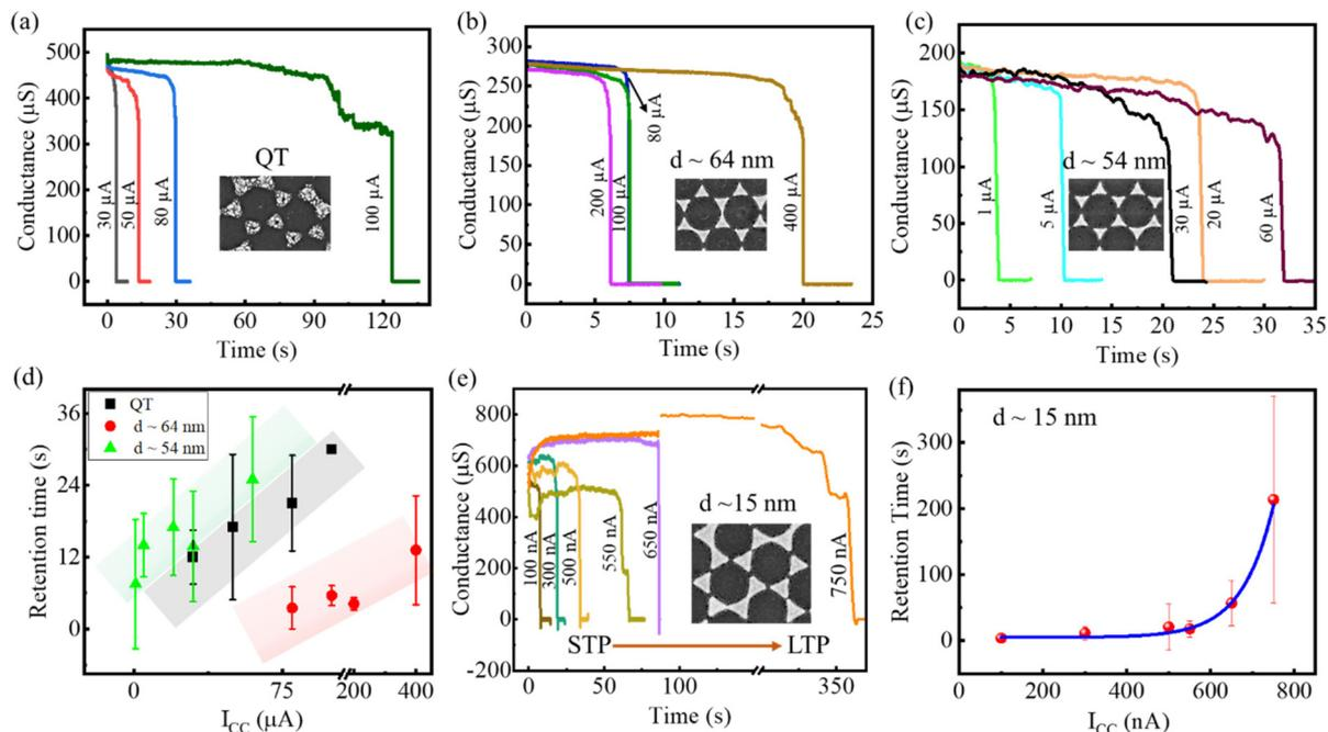
**Fig. 4** Memory retention and STP to LTP transition as a function of  $I_{CC}$  for devices having (a) QT structure, (b)  $d \sim 64$  nm (c)  $d \sim 54$  nm. Retention time variation as a function of  $I_{CC}$  for (d) QT structure,  $d \sim 64$  nm, and  $d \sim 54$  nm. (e) STP to LTP transition of conductance at low  $I_{CC}$  (nA) of  $d \sim 15$  nm device and its (f) retention time versus  $I_{CC}$  plot.
