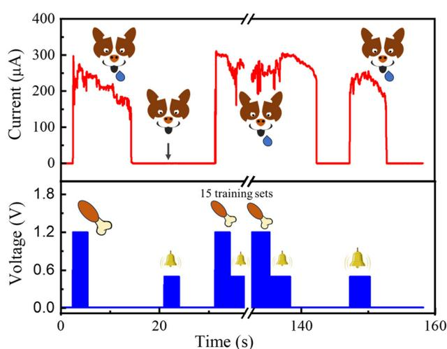
**Fig. 5** Emulation of classical conditioning using the device subjected to an appropriate training set of food (1.2 V) and bell (0.5 V) pulses. Before training, the response was observed only with the food pulse, whereas it was absent for the bell pulse. After training with 15 consecutive sets of food and bell pulses, the device responded to the bell pulse alone thereby mimicking associative learning.
