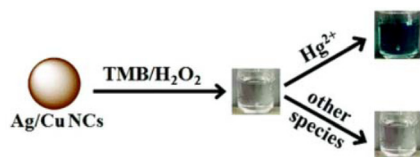
Fig. 13 Schematic representation of mercury(II) sensing with Ag/CuCNs. Reproduced from ref. 149, with permission from Anal. Methods , Copyright 2021.
