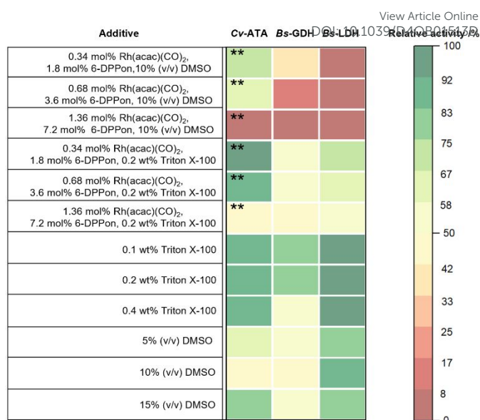
Figure 4: “Heat-map” depicting the relative activities of Cv -ATA, Bs -GDH, and Bs -LDH in the presence of various additives. The relative activity is defined as (volumetric activity with additive) related to (volumetric activity without additive) and represented by a colour gradient. Green indicates a high relative activity, while red indicates low relative activity. The [Rh(acac)(CO) 2 ] and 6-DPPon concentrations are expressed as mol% relative to a 50 mM substrate concentration.
