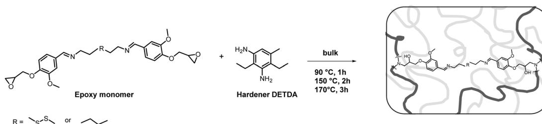
Fig. 3 Synthesis of epoxy SDBB/DETDA and DDBB/DETDA-based vitrimers.
