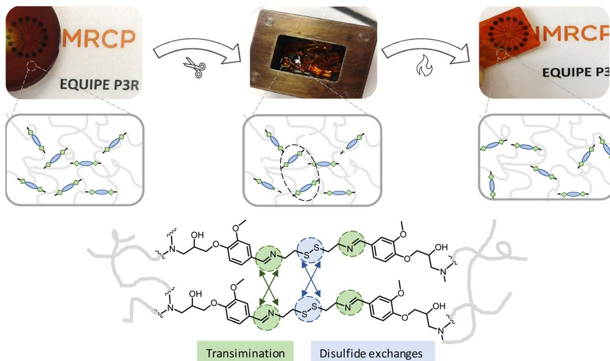
**Fig. 8** Example of reprocessing experiment via compression moulding of DDBB<sub>0.30</sub>DGEBA<sub>0.70</sub>/4AFD formulation in a hot press at 170 °C.
