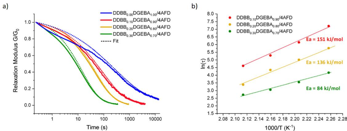
**Fig. 7** (a) Stress relaxation experiments at 190 °C of DDBB<sub>x</sub>DGEBA<sub>y</sub>/4AFD formulations with  $x$  ranging from 0 to 0.30 and  $y$  from 1.00 to 0.70 and (b) corresponding Arrhenius dependence.
