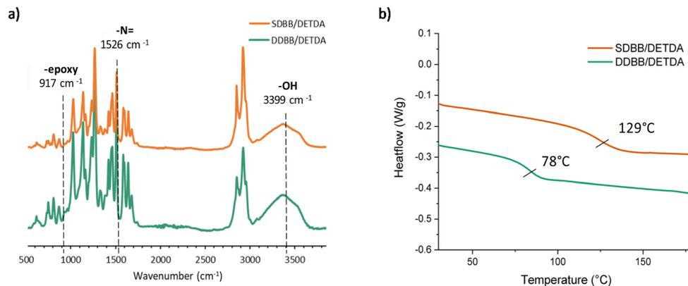
Fig. 4 (a) FTIR spectra of SDBB (orange) and DDBB (green) after curing (b) DSC thermograms of SDBB and DDBB after curing.
