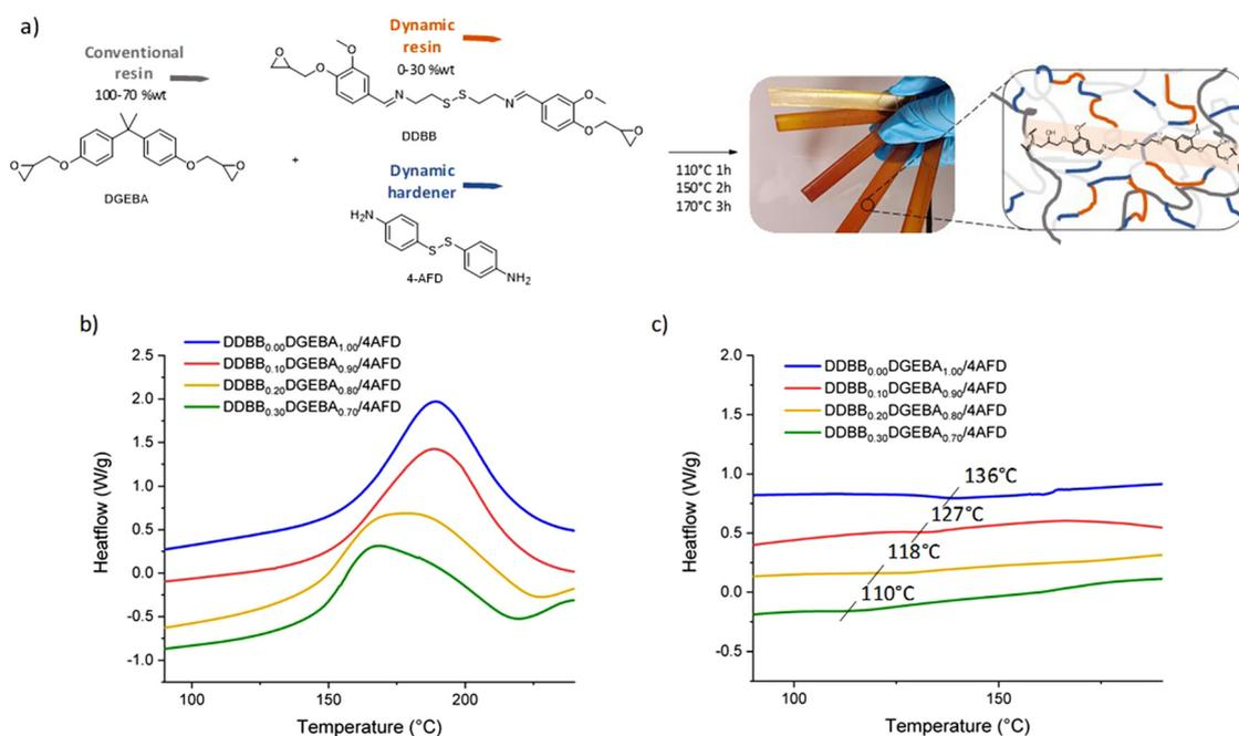
**Fig. 6** (a) Synthesis of DDBB<sub>x</sub>DGEBA<sub>y</sub>/4AFD-based epoxy vitrimers (b) DSC thermograms obtained at a heating rate of  $10 \text{ °C min}^{-1}$  for DDBB<sub>x</sub>DGEBA<sub>y</sub>/4AFD mixtures (c) corresponding  $T_g$  obtained during a second heating ramp at  $10 \text{ °C min}^{-1}$ .
