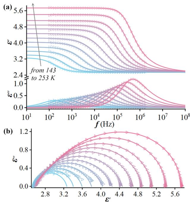
**Fig. 4** Frequency-dependent  $\epsilon'$  and  $\epsilon''$  for **2** at selected temperatures from 143 to 253 K in an increasing step of 10 K (a), and the Cole–Cole diagrams are plotted as a series of arcs to show the relationship between  $\epsilon'$  and  $\epsilon''$  (b). Solid curves represent the fit of the experimental data to the Havriliak–Negami equation.
