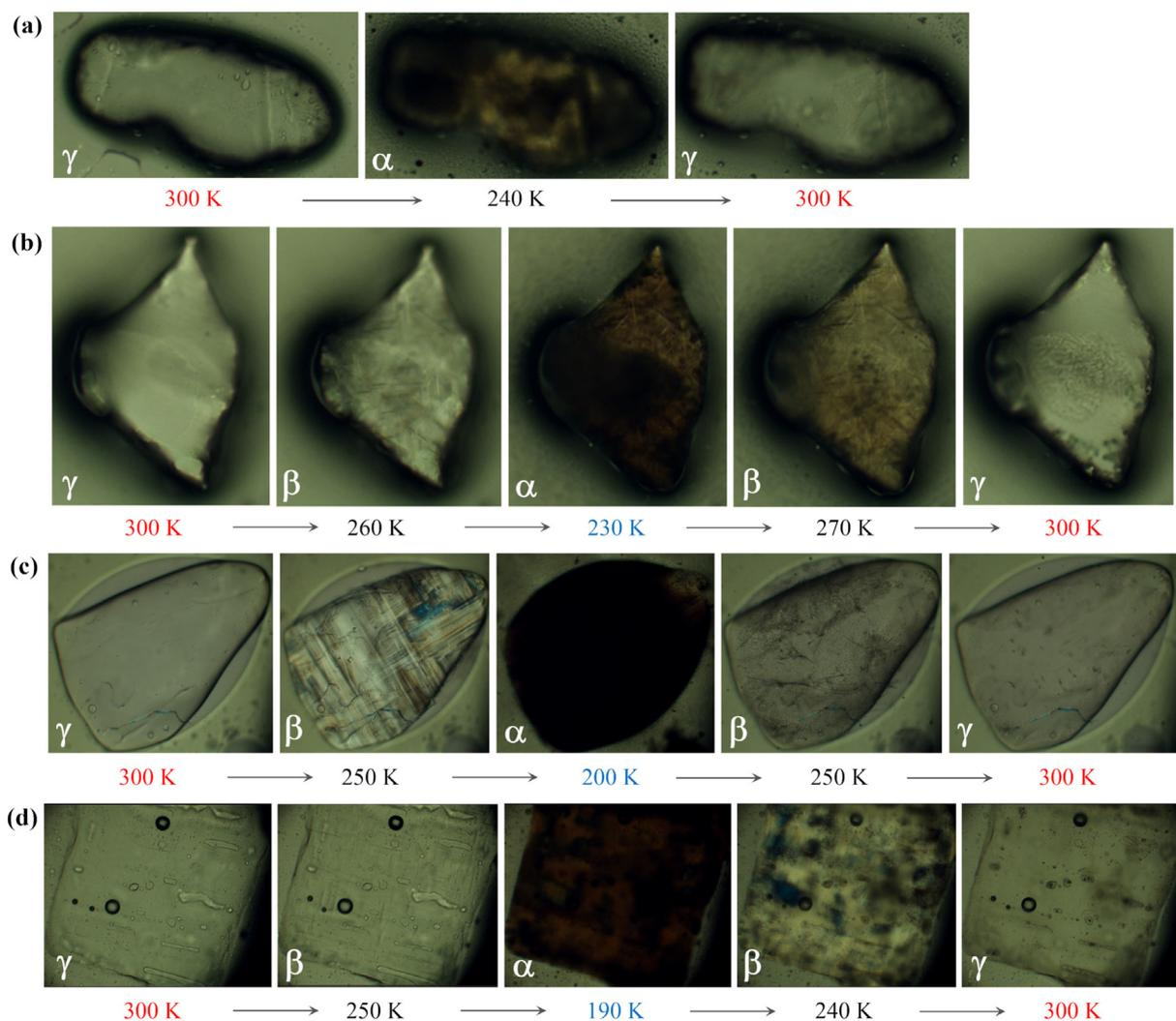
**Fig. 6** Variable-temperature evolution of the ferroelastic domains for **1** (a), **2** (b), **3** (c) and **4** (d), respectively, observed under polarization microscope. Crystal sizes:  $1.4 \times 0.4 \times 0.2$  mm for **1**,  $1.6 \times 0.7 \times 0.3$  mm for **2**,  $2.2 \times 1.3 \times 0.5$  mm for **3**, and  $2.5 \times 2.3 \times 0.3$  mm for **4**.
