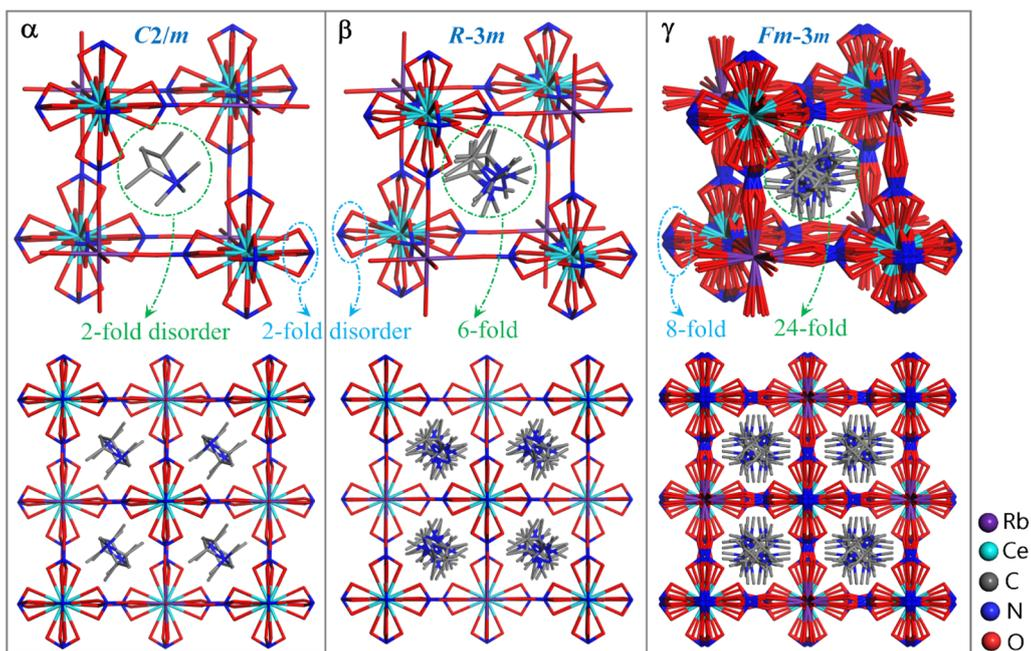
**Fig. 2** Cage units and packing diagrams of **2** at 173 K ( $\alpha$  phase), 273 K ( $\beta$  phase), and 293 K ( $\gamma$  phase), respectively. The  $(i\text{-PrNHMe}_2)^+$  and  $\text{NO}_3^-$  ions exhibit varying degrees of disorder in all phases. H atoms are omitted for clarity.
