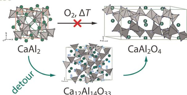
**Mechanistic studies on the formation of ternary oxides by thermal oxidation of the cubic laves phase CaAl<sub>2</sub>**
