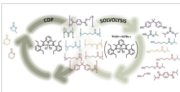
**Divergent methods for polyester and polycarbonate depolymerization with a cobalt catalyst**
