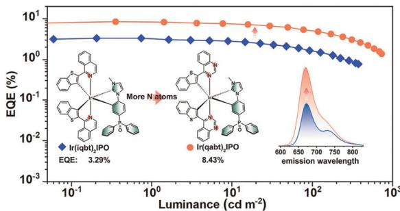
**Boosting the efficiency of deep-red Ir(III) complexes by modulating nitrogen atoms for high-performance OLEDs**
