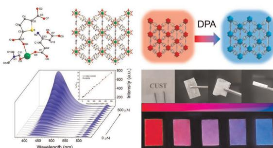
**Eu<sup>3+</sup>-MOF fluorescence sensor based on a dual-ligand strategy for visualised detection of an anthrax biomarker 2,6-pyridine dicarboxylic acid**
