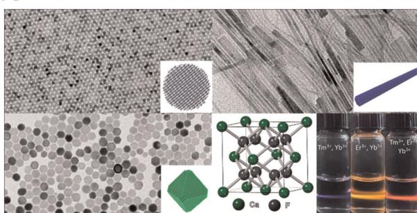
**Shape-controlled synthesis and self-assembly of highly uniform upconverting calcium fluoride nanocrystals**
