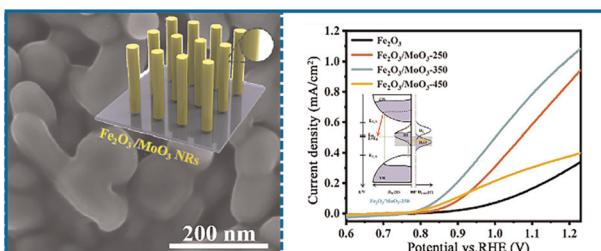
**Boosting the photoelectrochemical water splitting of  $Fe_2O_3$  by surface-state regulation**
