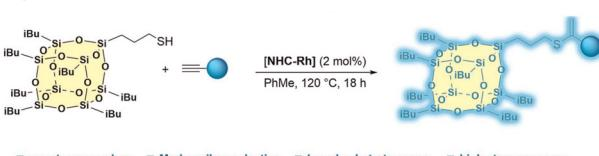
**Highly effective synthesis of mercapto-functionalized cubic silsesquioxanes as the first step in designing advanced nano-delivery systems**
