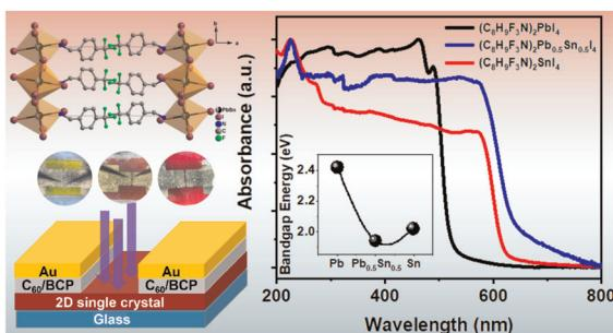
**Centimeter-sized novel two-dimensional organic lead–tin mixed iodide single crystals for efficient photodetector applications**
