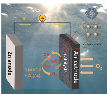
**Interfacial engineering of cobalt phosphide heterostructures confined in N,P-doped carbon for efficient bifunctional electrocatalysis in Zn-air batteries**
