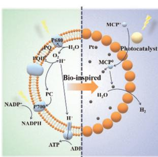
**Bioinspired electron carrier mediated transmembrane photocatalytic hydrogen evolution in silica colloidosomes**
