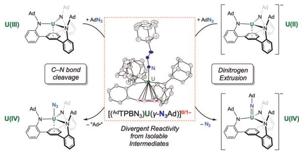
**Divergent reactivity of U(III) and U(II) complexes with organoazides via isolable diazenylimido intermediates**
