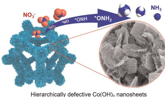
**Deep self-reconstruction of  $\text{CoF}_2$  to hierarchically defective  $\text{Co}(\text{OH})_2$  nanosheets for electrocatalytic reduction of nitrate to ammonia**
