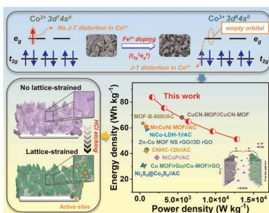
**Engineered iron-doped MOF nanosheets: acid-induced lattice strain for enhanced rate performance in asymmetric supercapacitors**
