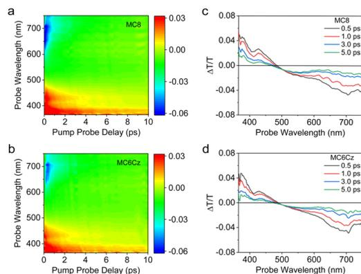
Fig. 2 Transient absorption (TA) analysis of **MC8** and **MC6Cz** films. TA contour plots of **MC8** (a) and **MC6Cz** (b). (c) and (d)  $\Delta T/T$  spectra of **MC8** and **MC6Cz** films from 0.5 to 5.0 ps pump-probe delay.
