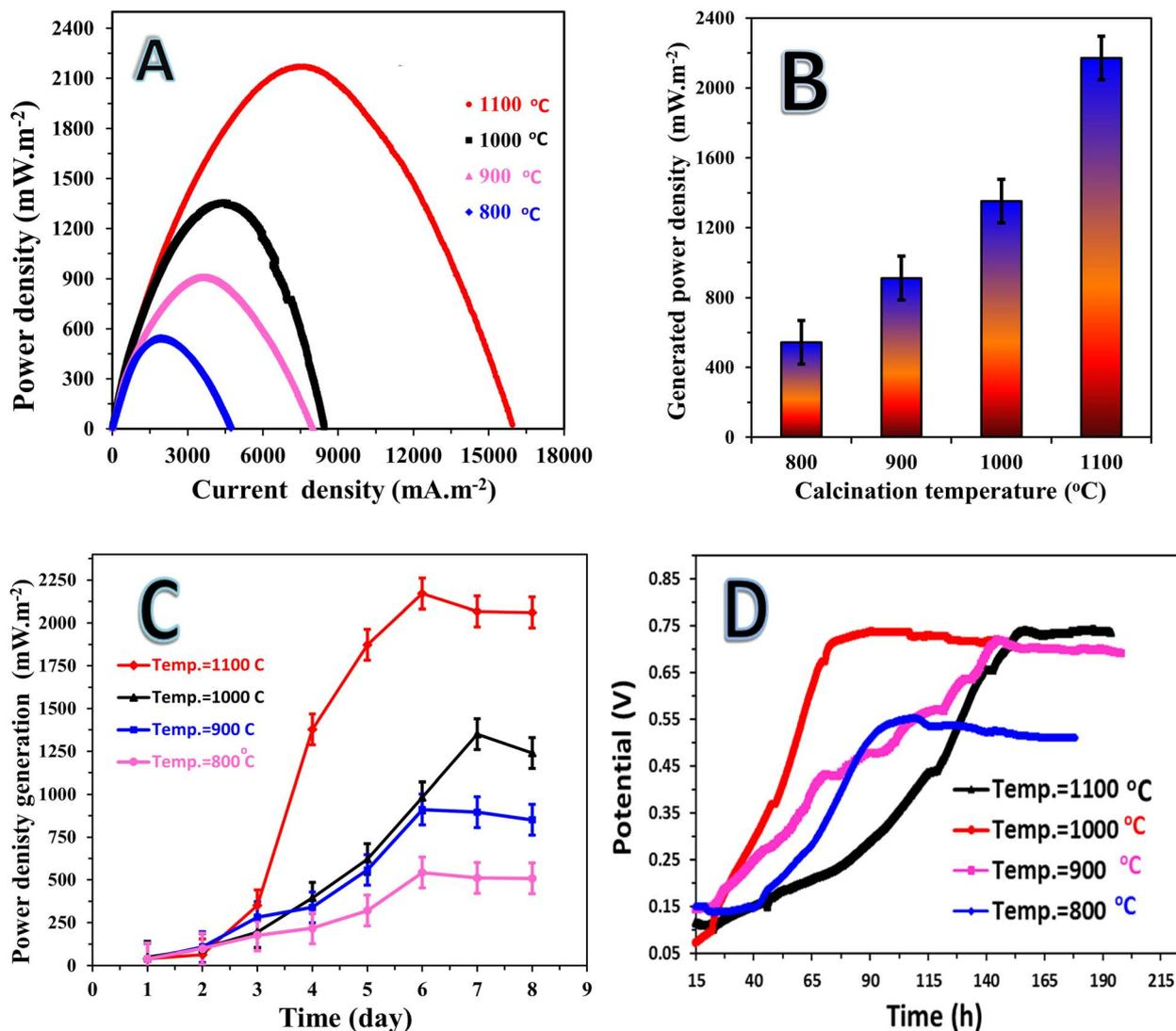
Fig. 6 Influence of mango seed calcination temperature on the performance of NaAc ( $5 \text{ g L}^{-1}$ )/sewage wastewater-based microbial fuel cells. (A) Polarization curves of the assembled microbial fuel cells, (B) maximum generated power densities at different calcination temperatures, (C) influence of running time on the generated power, and (D) change in the open cell potential with respect to time.
