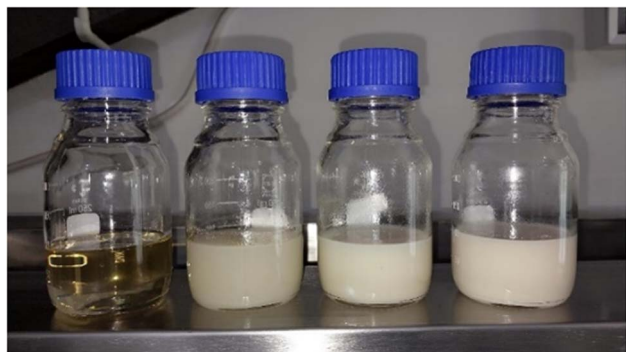
Fig. 3 Dope solution PSf and PSf/PPs 1, 5, and 10 wt%.
