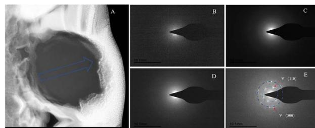
**Fig. 14** SAED analysis of section S1. (A) HAADF image of cross-section S1, with selected area diffraction indicated by the blue arrow. (B–E) Selected area diffraction patterns from the regions indicated by arrows in image (A); among these, (B–D) exhibit characteristics of amorphous materials, and in conjunction with elemental analysis, are presumed to represent ACC; the polycrystalline rings in image (E) correspond to the (100) and (300) crystal planes of vaterite.
