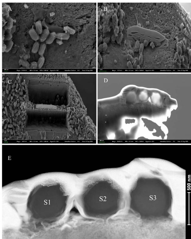
**Fig. 12** SEM images of FIB sectioning process and HAADF-STEM image of the selected calcified bacterial particles. (A) SEM image of the rod-shaped minerals cut by FIB; (B) Pt embedding; (C) process of FIB milling and sample extraction; (D) thin section cut to a thickness of 50–60 nm, containing three rod-shaped mineral particles; (E) HAADF (High-Angle Annular Dark-Field) images, with three sections labeled as S1, S2, and S3.
