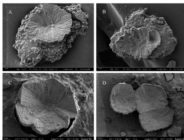
**Fig. 11** Concave-type morphologies of carbonate minerals templated by bacterial biofilms. (A and B) Represent the morphology of concave-type minerals found in samples from the 10th and 16th days, respectively, with a significant presence of calcified bacteria and biofilms at the bottom. (C and D) Represent the morphology of concave-type minerals observed in samples from the 25th and 30th days, respectively.
