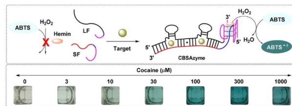
Fig. 2 Working mechanism and the chromogenic catalysis performance of the CSBAzyme. Reprint from ref. 43, with permission. Reprinted (adapted) with permission from Anal. Chem. , 2019, 91(11), 7199–7207. Copyright 2019 American Chemical Society.
