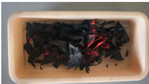
Fig. 1 Pyrophoric KOH-activated electrospun PAN-based carbon nanofibres during exposure to ambient air directly after the simultaneous carbonisation and KOH activation. A red glowing of the carbon nanofibres can be observed (a Video of the glowing is attached as ESI†).
