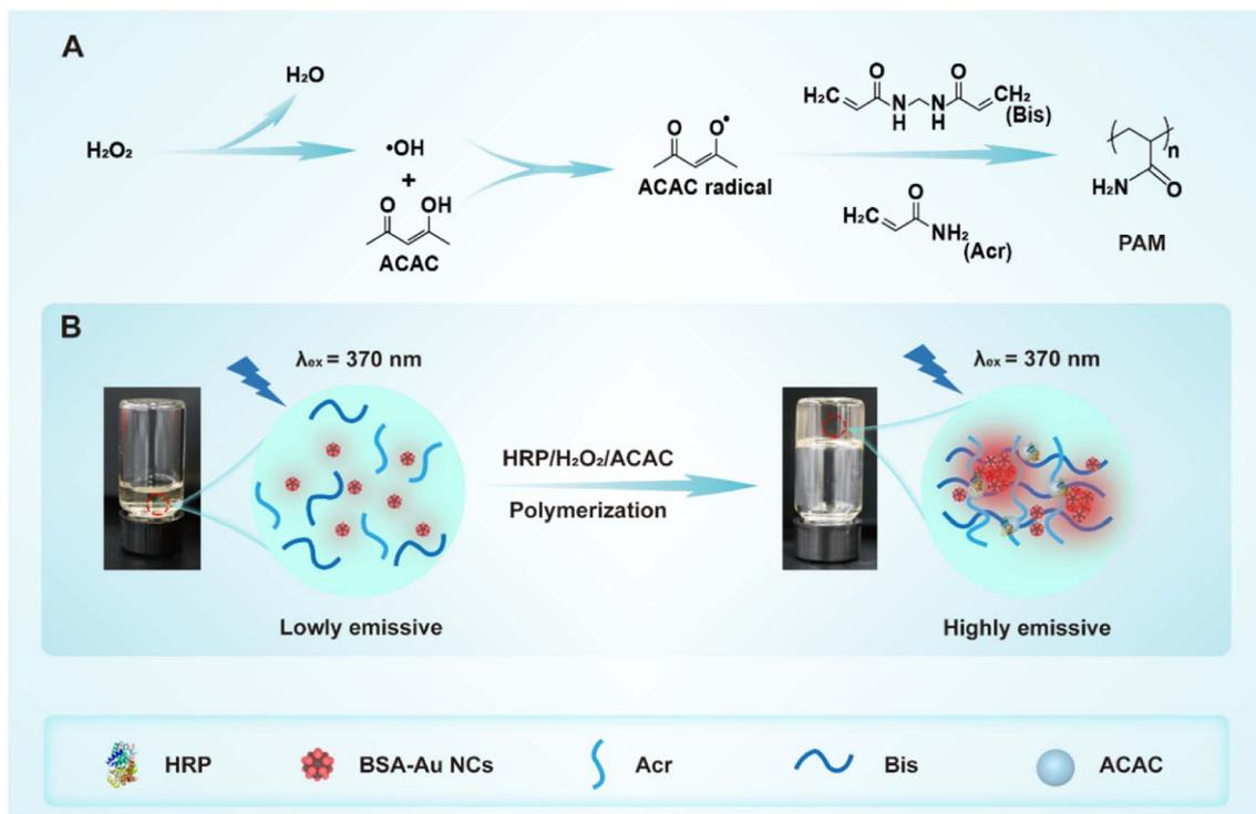
**Scheme 1** Schematic illustration of (A) Acr-Bis polymerization catalyzed by HRP/H<sub>2</sub>O<sub>2</sub>/ACAC ternary initiation system and (B) the polymerization of Acr-Bis causes AIE phenomenon of BSA-Au NCs.
