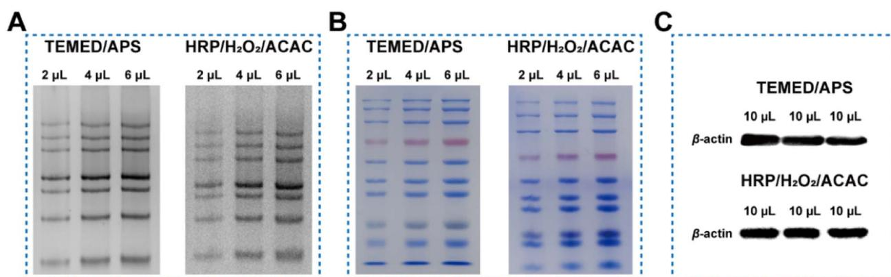
Fig. 4 Verification of the electrophoretic function of polyacrylamide gels catalyzed by HRP/ $\text{H}_2\text{O}_2$ /ACAC. Different concentration of DNA marker (A) and protein marker (B) were analyzed by performing electrophoresis using 10% polyacrylamide gels catalyzed by TEMED/APS (left) and HRP/ $\text{H}_2\text{O}_2$ /ACAC (right). (C) Western blot analysis of  $\beta$ -actin separated by the two kinds of polyacrylamide gel electrophoresis.
