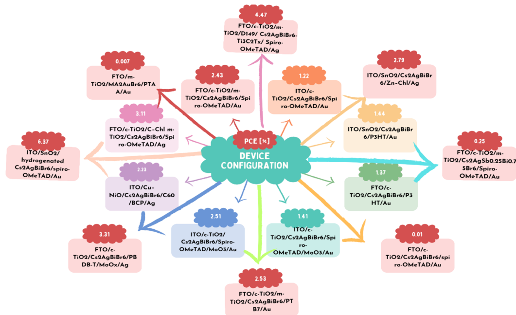
Fig. 15 Device architecture and photovoltaic parameters of HDP-based solar cells.
