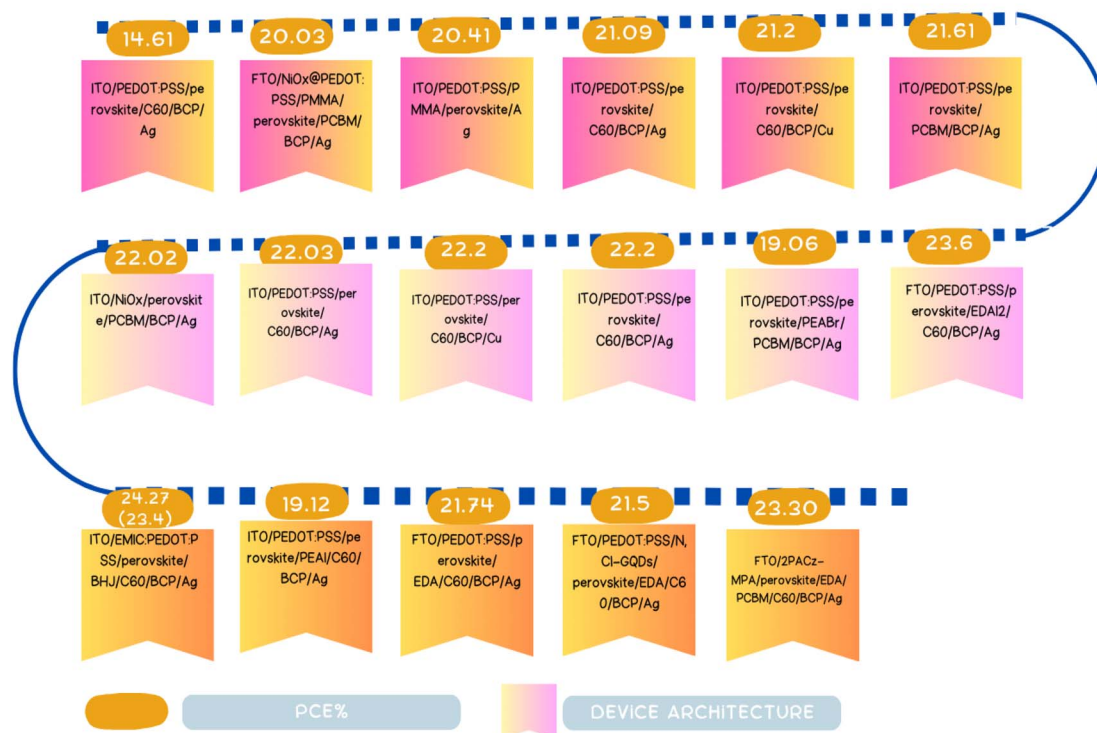
Fig. 11 Recent device performance of tin-lead mixed PSCs.
