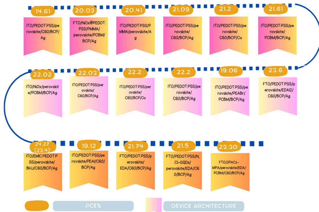
Fig. 11 Recent device performance of tin-lead mixed PSCs.
