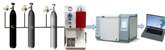
Fig. 2 Adsorption device of Na-X for a low concentration of CO 2 .
