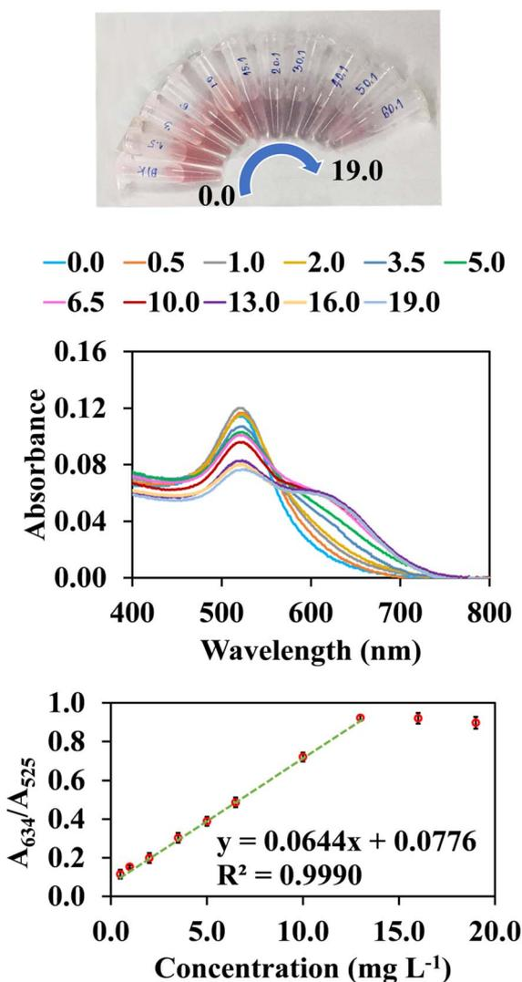
Fig. 9 Colorimetric changes, UV-vis spectra and their correlation with absorbance ratios ( $A_{634}/A_{525}$ ) and final concentrations of hydrolyzed cypermethrin (0.5–19.0 mg L<sup>-1</sup>).
