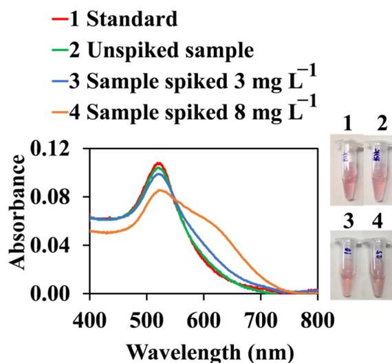
Fig. 10 Color images and UV-vis absorption spectra of AuNPs@Cyst for cypermethrin standard, unspiked sample and samples spiked with 3 and 8 mg L<sup>-1</sup> of cypermethrin for recovery test.
