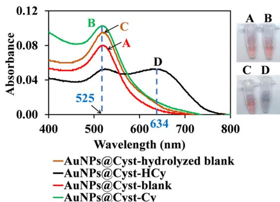
Fig. 3 UV-vis spectra of (A) AuNPs@Cyst blank, (B) AuNPs@Cyst-Cy, (C) AuNPs@Cyst-hydrolyzed blank, and (D) AuNPs@Cyst-HCy at 50 mg L<sup>−1</sup> cypermethrin. The inset shows the colorimetric responses corresponding to the UV-vis spectra.
